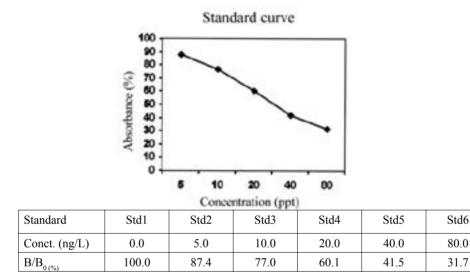
Fig. 1. Calibration curve of a RIDASCREEN® AFM1 kit and reference values
